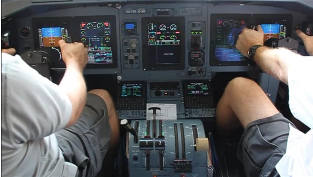
Figure 2: Still image from video of on-ground pitch disconnect testing carried out on VH-FVR following the occurrence. The right control column was held fully forward while the left control was pulled back. The image is just before the pitch uncoupling mechanism activated. Note the difference between the left and right control column positions. The left control column is about halfway through its full travel, while the right control column is at the forward limit.
