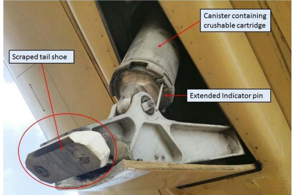
Figure 1: Damage to tail skid
