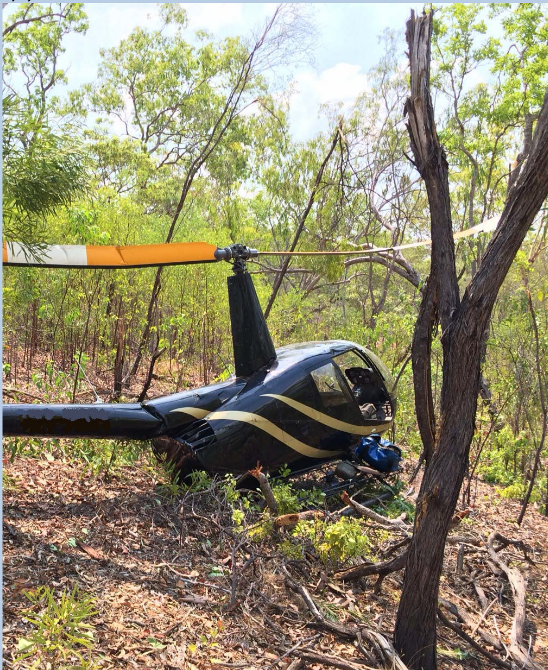
Damage caused by hard landing after a Whistling Kite struck the tail rotor of an R44. Source: Reporter
