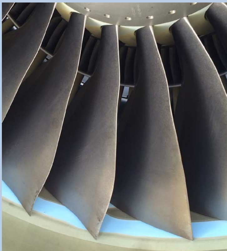
Fan blade damage (lower left of image) caused by ingesting a Cattle Egret. Source: Reporter
