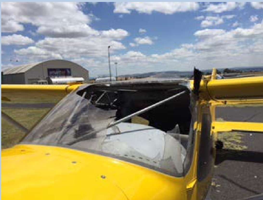
The result of an impact with a Wedge-tailed Eagle, showing where the animal penetrated the windshield of the Glasair Sportsman GS-2. Source: Reporter
