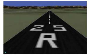
Figure 5: Synthetic vision runway display on approach (at low altitude)
