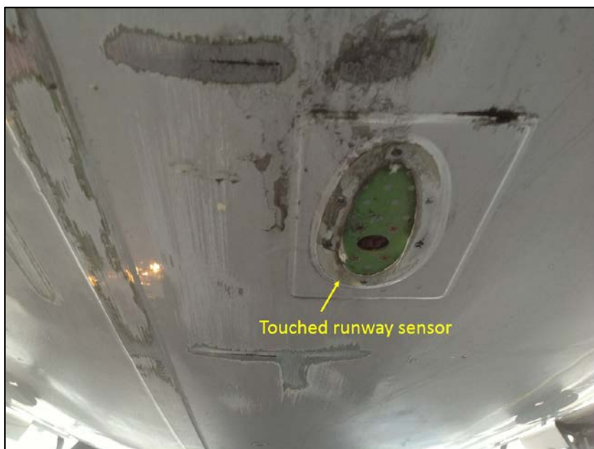
Figure 4: Damage to tail section of VH-QOS (looking aft)
