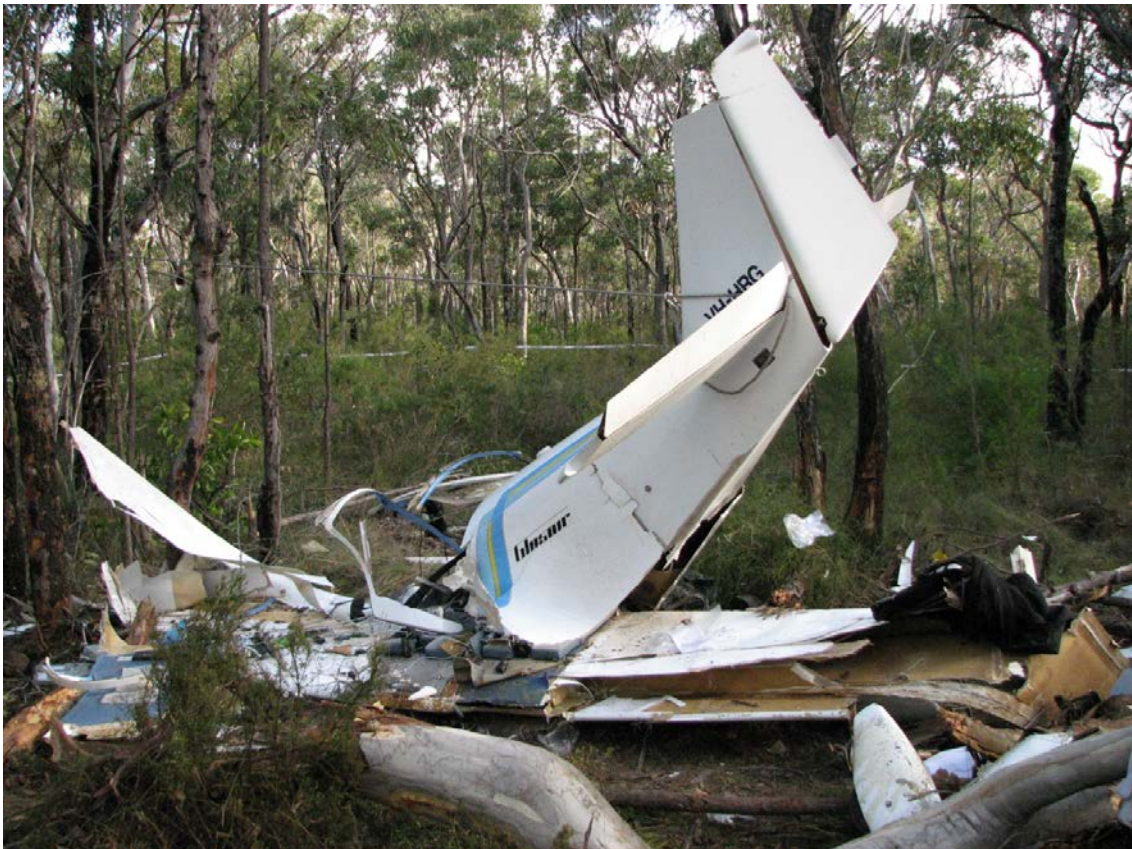
Figure 2: Aircraft wreckage. Note that the tail empennage is secured in an elevated position by being tied off to a nearby tree
