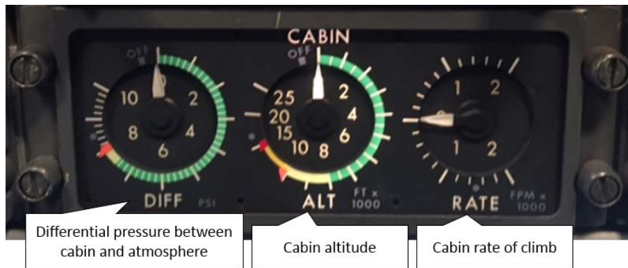
Figure 1: F28 cabin pressure gauges
