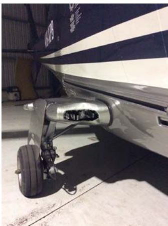
Figure 2: Damage to right landing light of VH-XPB
