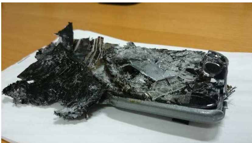
Figure 3: Crushed PED after removal from seat
