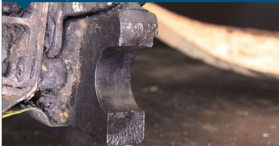
Figure 10: Outboard view of the fractured lower attachment fitting at the left wing main spar interconnection
