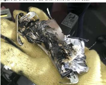
Figure 2: Crushed PED after removal from seat
