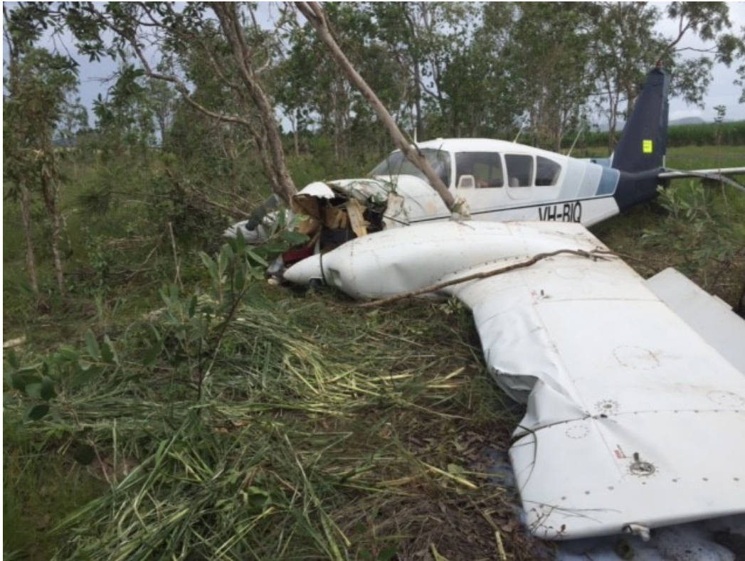
Figure 1: Accident site showing damage to VH-BIQ
