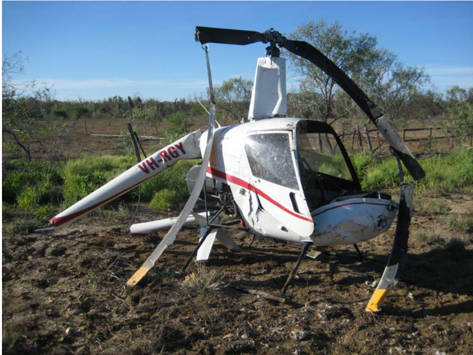
Figure 2: Damage to VH-RGY (after removal from accident site)
