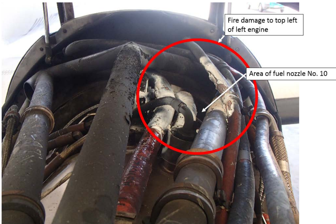
Figure 1: Fire damage to the left engine
