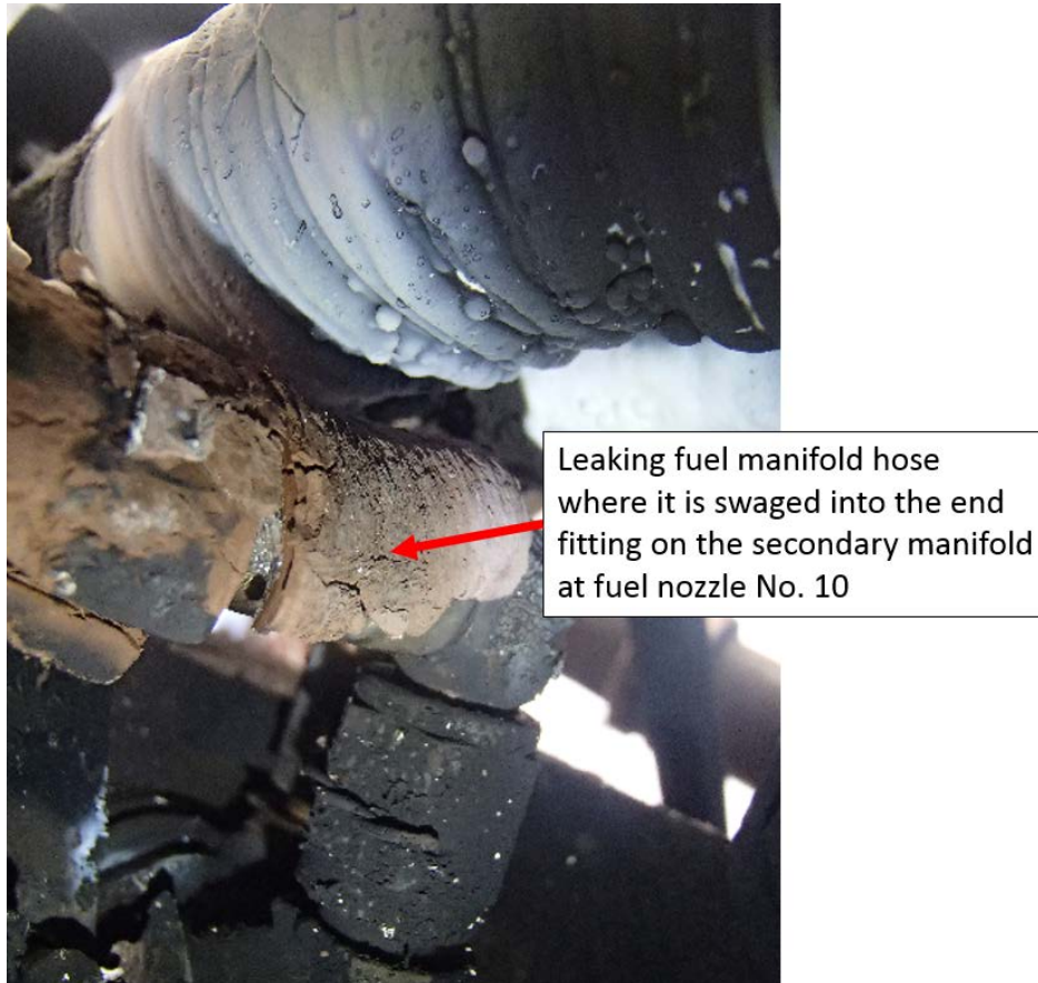
Figure 2: Leaking flexible fuel manifold hose
