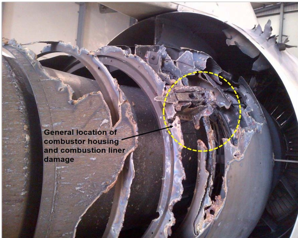
Figure 1: Right side of the No.2 engine showing the fire damage to the combustor housing and liner (looking forward)
