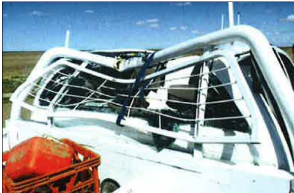
Figure 3: Rear view showing damage to the Hilux headboard
