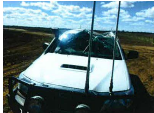
Figure 4: Roof structure damage on passenger side
