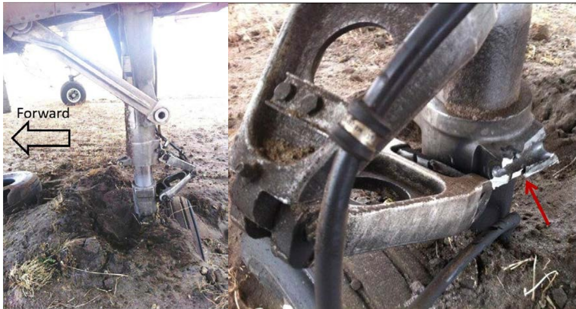
Figure 1: Damage to the left MLG
