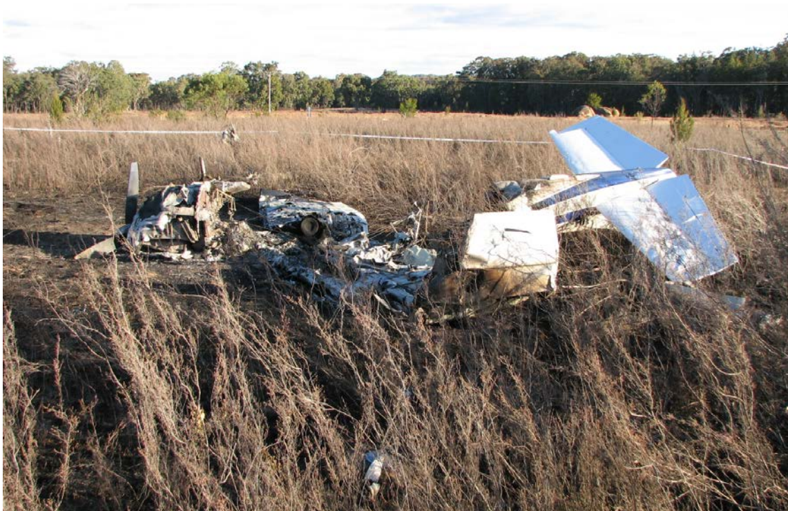
Figure 4: Aircraft wreckage showing the tail empennage inverted to the right and the propeller visible on the left (looking south-south-west)
