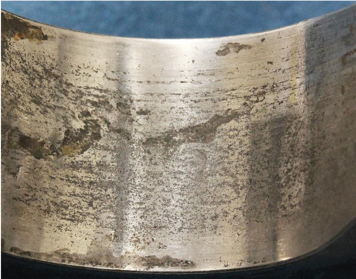
Figure B15: Fractured lug bore exhibiting extensive corrosion pitting
