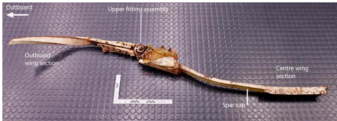
Figure B2: Left wing main spar upper fitting and spar cap – as recovered from the accident site
