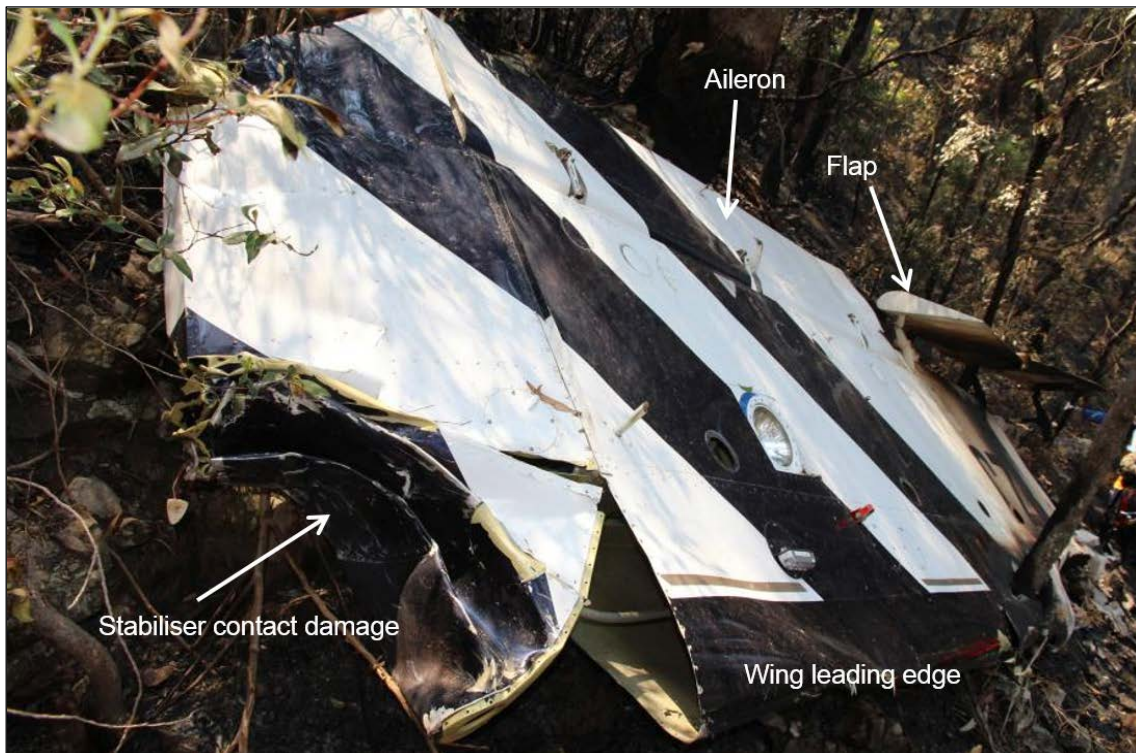
Figure 11: Left outboard wing, looking from the wingtip inboard and showing the lower surface of the wing
