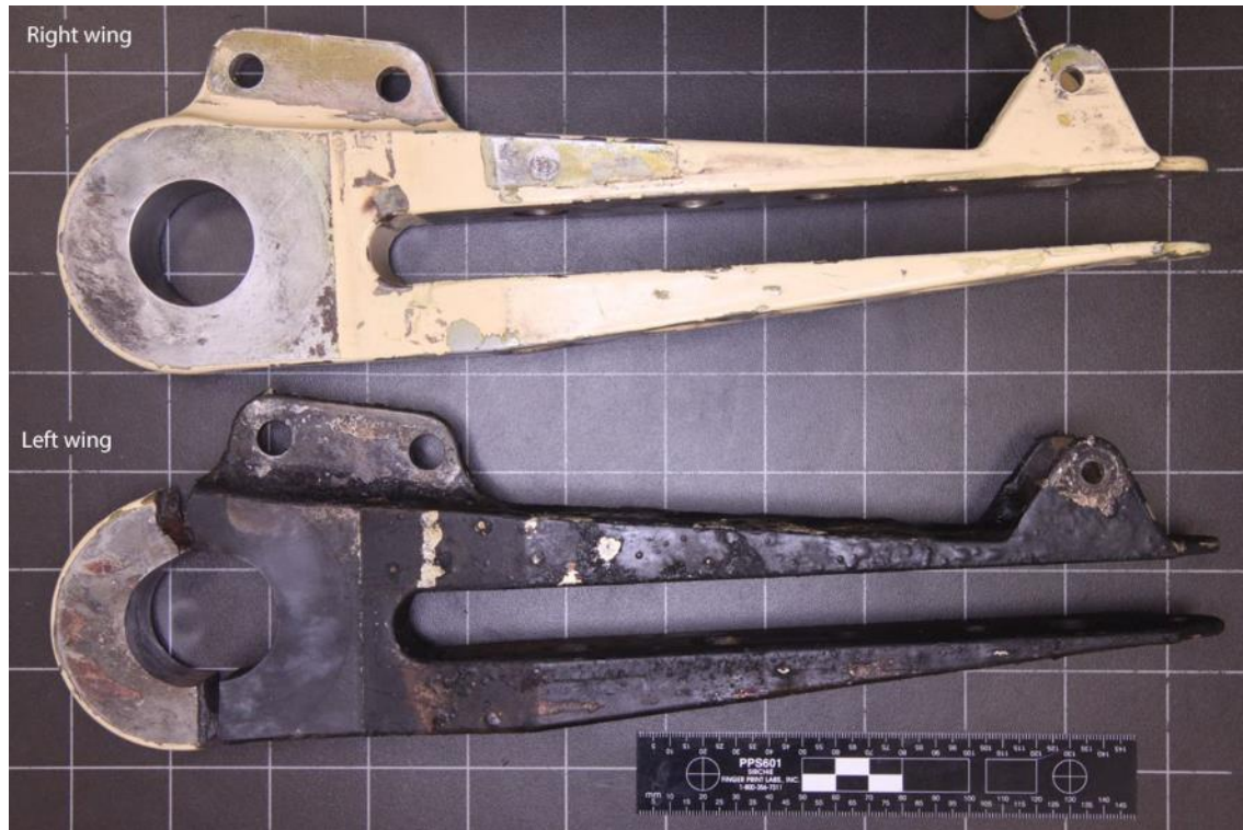
Figure B8: Comparison of the left and right main spar lower outboard attachment fittings from VH-TZJ (post disassembly)
