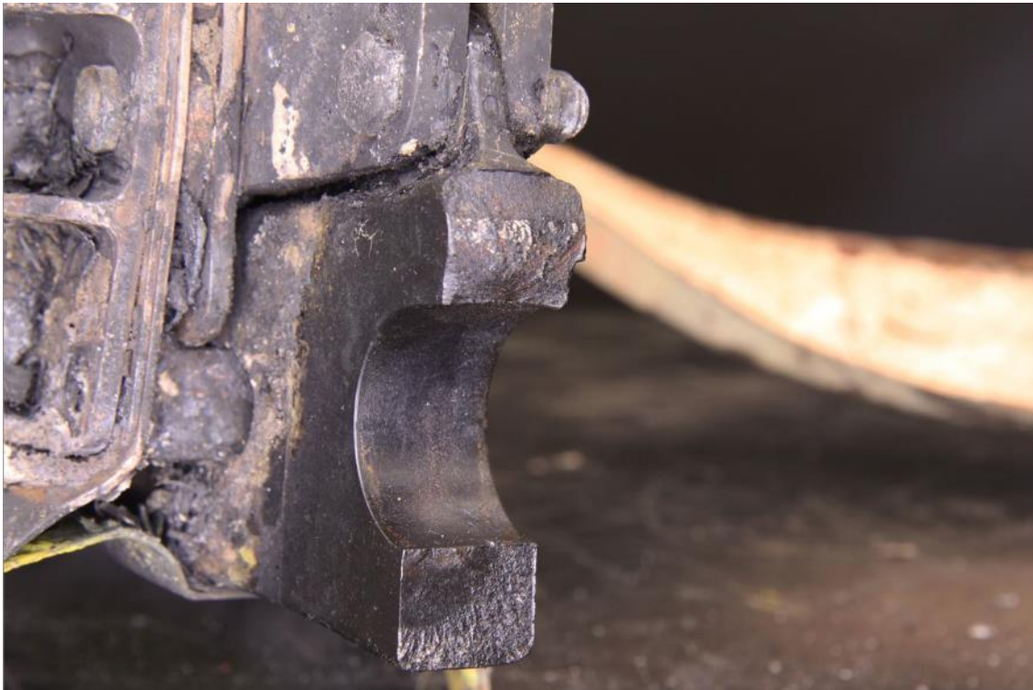
Figure B6: Outboard view of the fractured lower attachment fitting at the left wing main spar interconnection
