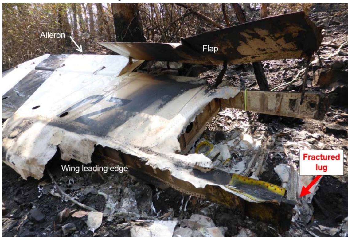
Figure 12: Left outboard wing from the inboard end showing fire damage and the fractured lower attachment lug
