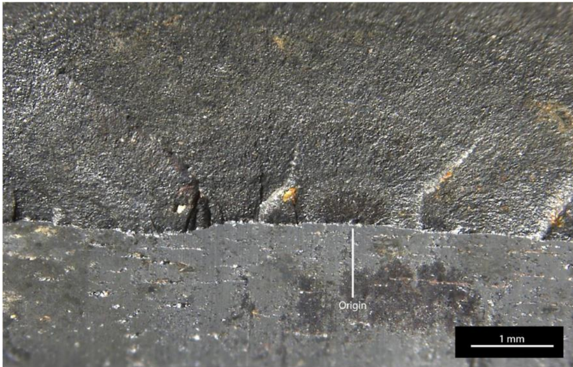
Figure B13: One of the fatigue crack origins (labelled) initiated from a corrosion pit within the bore of the fitting
