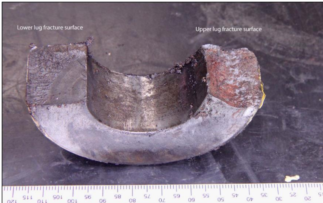
Figure B9: The fractured lug section from the left wing main spar outboard lower attachment fitting. The lug is shown uncleaned as disassembled
