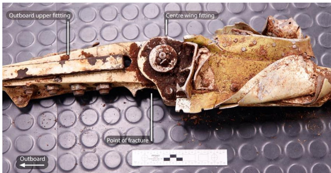
Figure B3: Left wing main spar upper attachment
