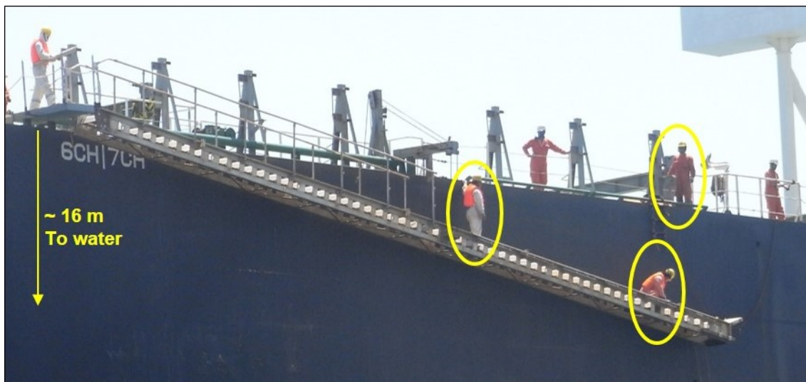
Figure 6: Crew rigging the accommodation ladder without fall protection and/or lifejacket
