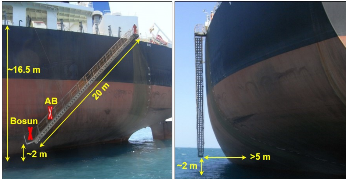
Figure 3: The accommodation ladder as rigged at the time of the accident showing distances and approximate positions of bosun and able seaman
