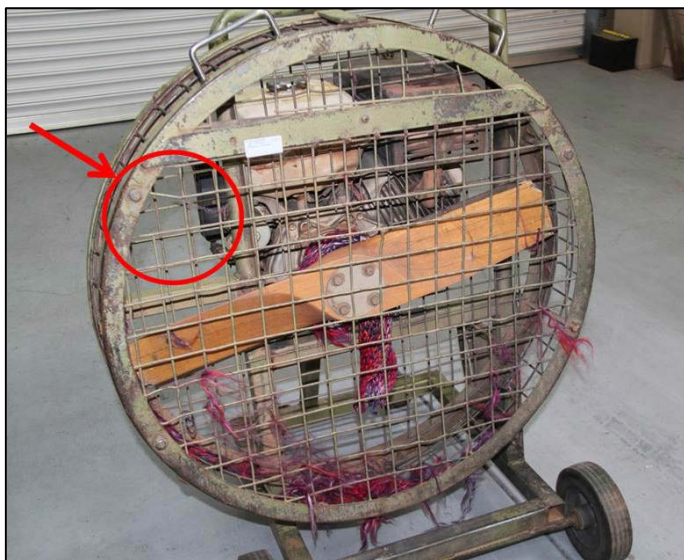
Figure 8: The cold-air inflation fan with remnants of the scarf (pre-existing minor cage damage highlighted)
