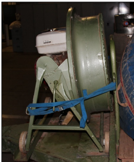
Figure 12: Shrouded fan design
