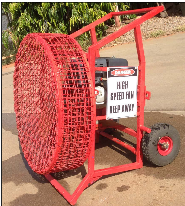
Figure 14: Modified fan guard with reduced mesh size
