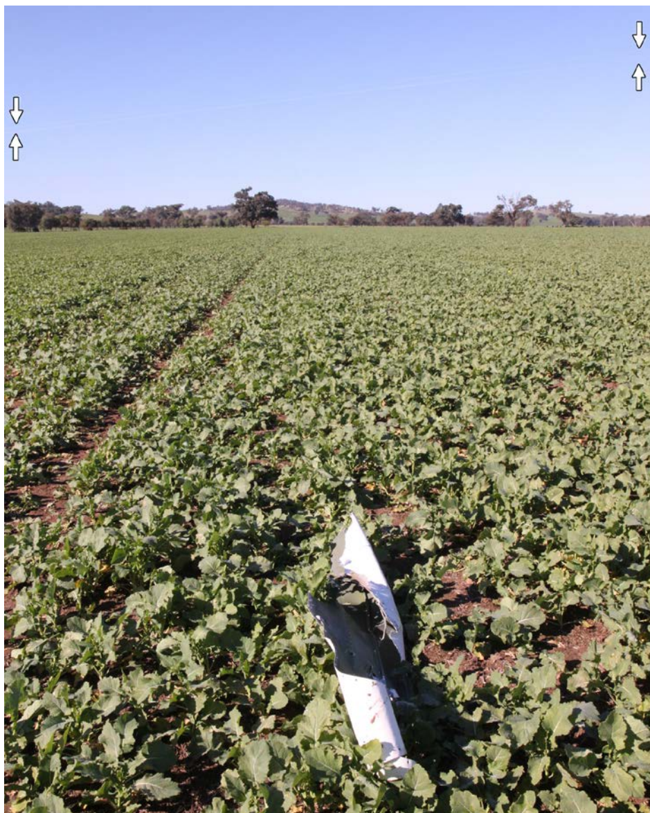
Figure 7: The powerline (electrical wires arrowed) looking back along the flight path. A piece of the leading edge skin from the left wing is also shown
