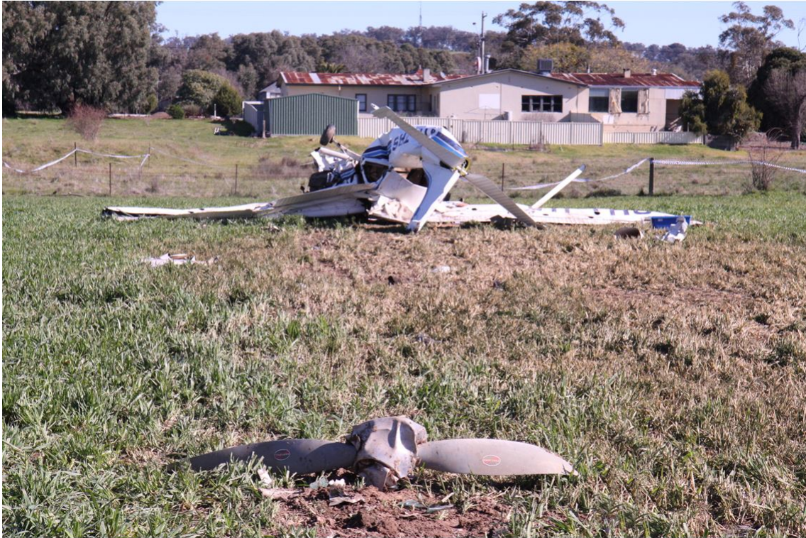
Figure 2: The aircraft impacted terrain near the Farmers Inn hotel. The aircraft was inverted at impact and the propeller separated from the engine
