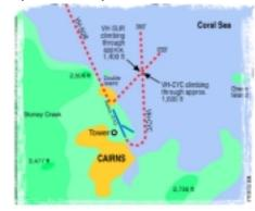
The Cessna had been cleared to execute a standard instrument departure and the Shorts commenced a missed approach. The missed approach and departure tracks at Cairns were within a 40 degree sector to the north east due to terrain constraints. The two aircraft crossed tracks at approximately 2 nm north east and were only able to avoid further conflict when they entered a clear area at the same time and the crews sighted each aircraft.
