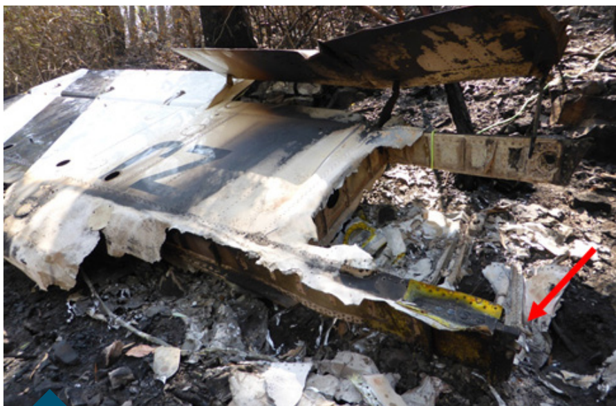
M18 Dromader outboard left wing (underside of wing visible, lower attach fitting arrowed)
