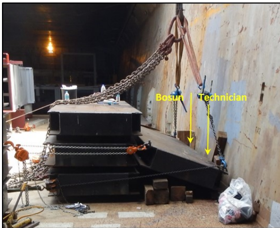
Figure 2: Fallen load spreader
