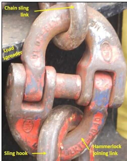
Figure 3: Hammerlock joining link
