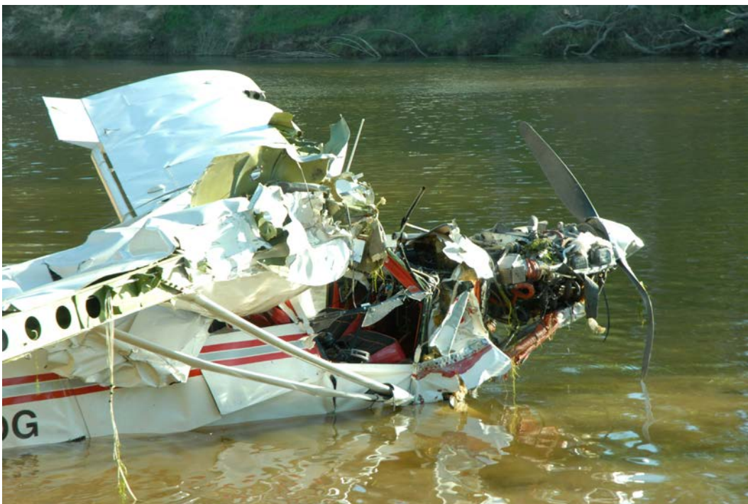
Figure 6: Damage to right wing and also in proximity to the right rear cabin door
