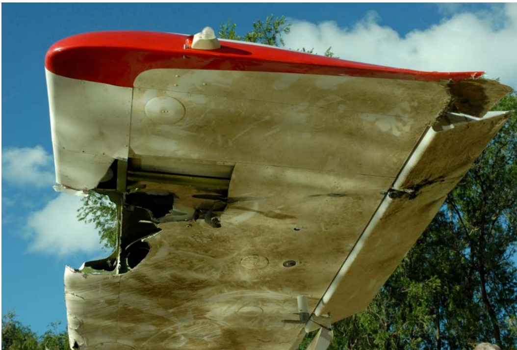
Figure 4: Damage to the left wing outboard leading edge
