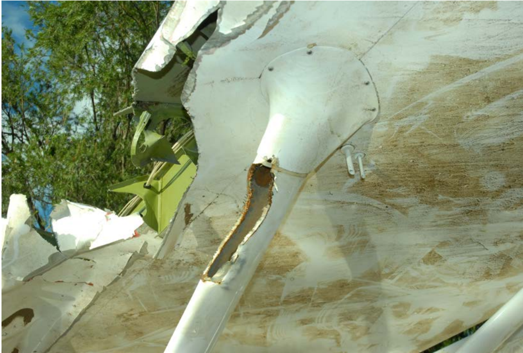
Figure 5: Damage to the left wing mid-section leading edge and wing support strut
