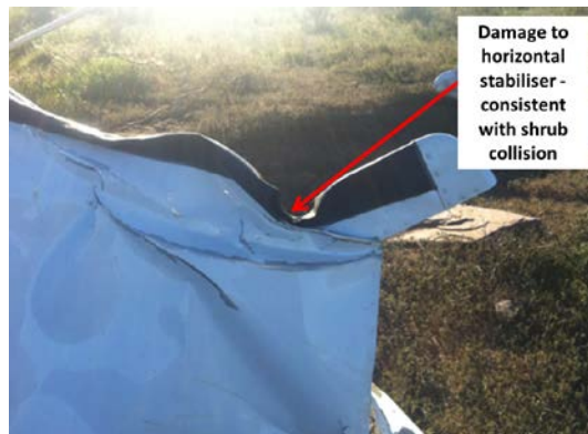
Figure 3: Damage to horizontal stabiliser
