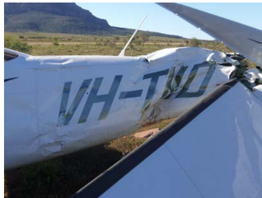
Figure 4: Rear fuselage and tail damage
