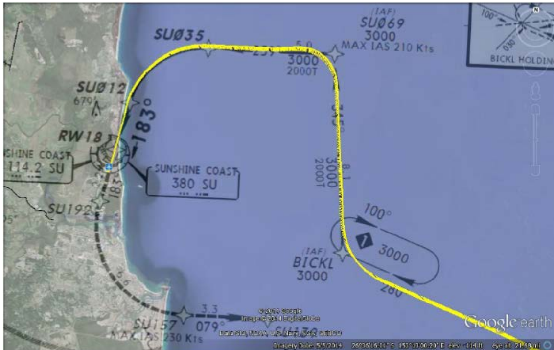
Figure 2: VH-VGJ track via the RNAV-X RWY 18 approach
