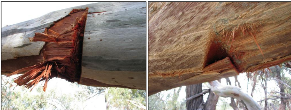
Figure 4: Propeller contact marks
