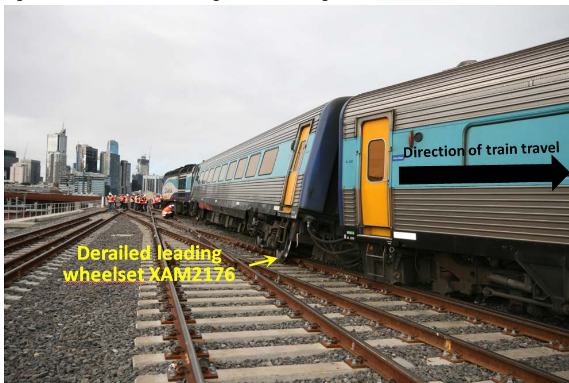
Figure 5: Photo – Derailed leading wheelset carriage XAM2176
