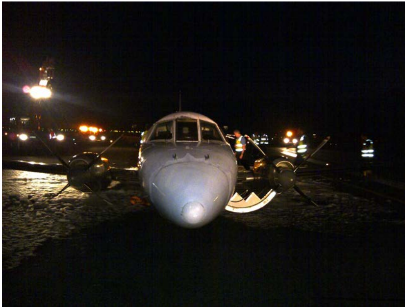
Figure 1: VH-UZA on runway 19 following the wheels-up landing
