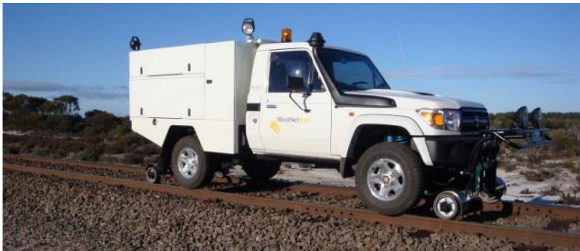
Figure 4: Non-elevation type rail guidance equipment fitted to a Toyota Landcruiser
