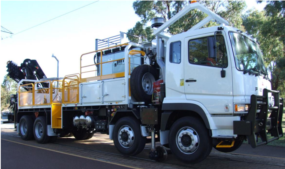
Figure 5: Elevation type rail guidance equipment fitted to a dual-rear-axle truck
