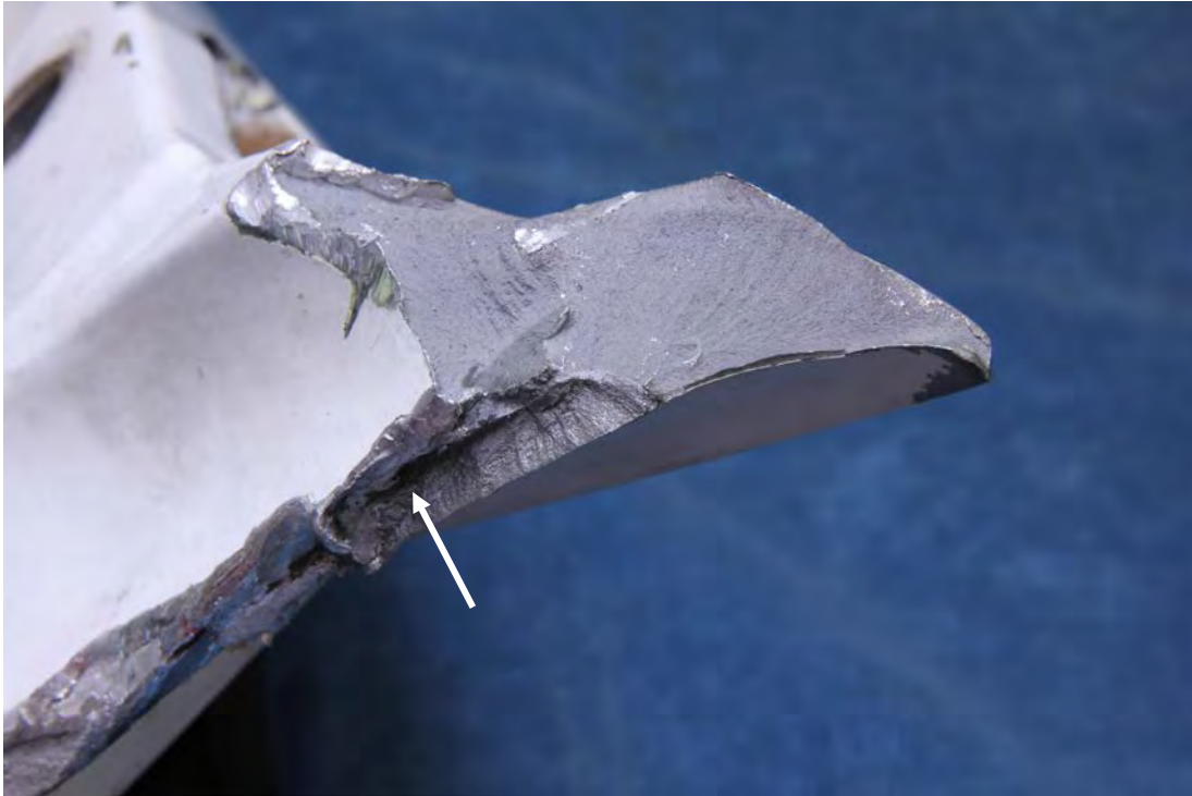
Figure A4: Inclined flange transition region of fracture (horizontal beam rear section) showing internal separation of the web (arrowed)
