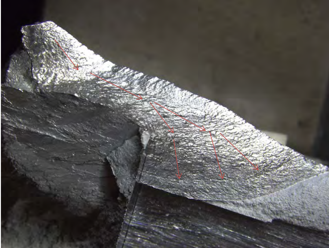
Figure A6: Intersection of central planar separation feature (piece shown in figure A5) with transverse progressive cracking (after sectioning). Arrows show direction of fatigue propagation
