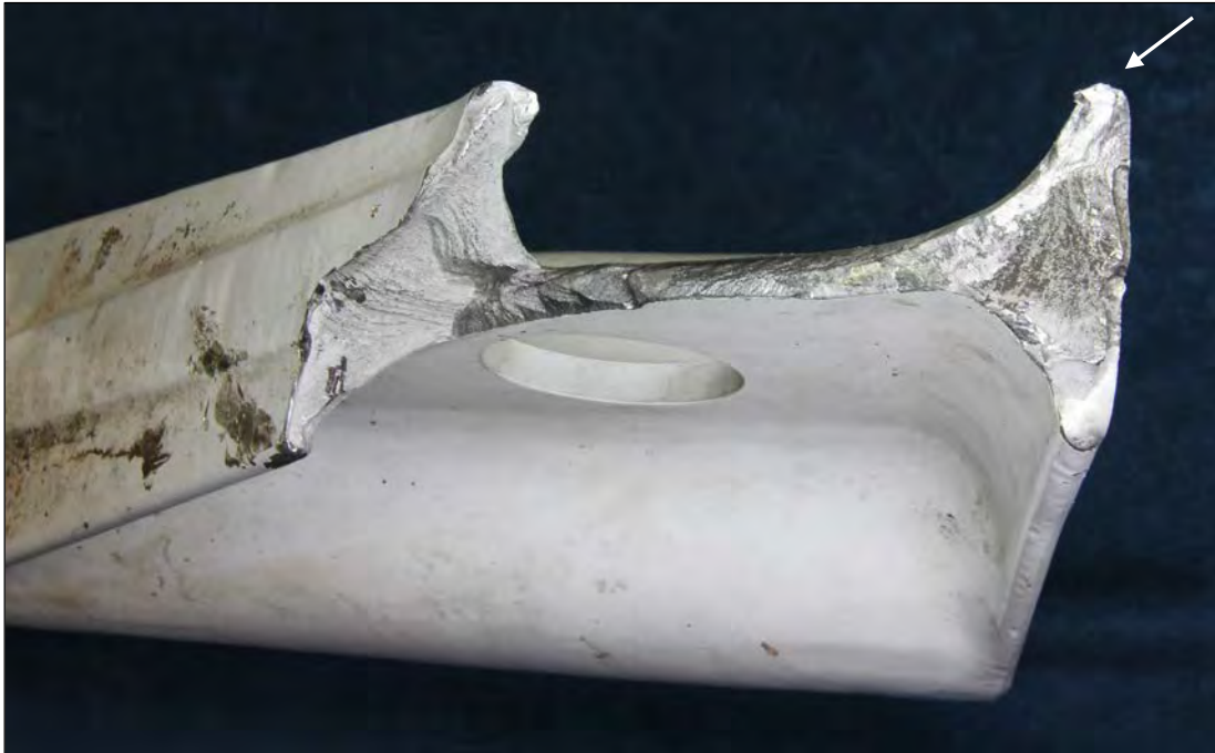
Figure A2: Fracture surface from vertical leg section – possible fatigue crack origin at damaged upper flange corner (arrowed)
