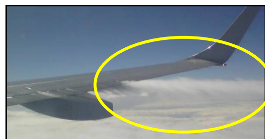
Figure 1: Photograph taken by cabin crew of vapours from right wing during descent
