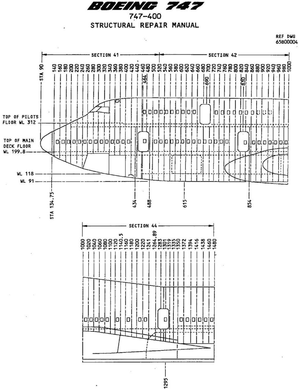
Fuselage Station Diagram
