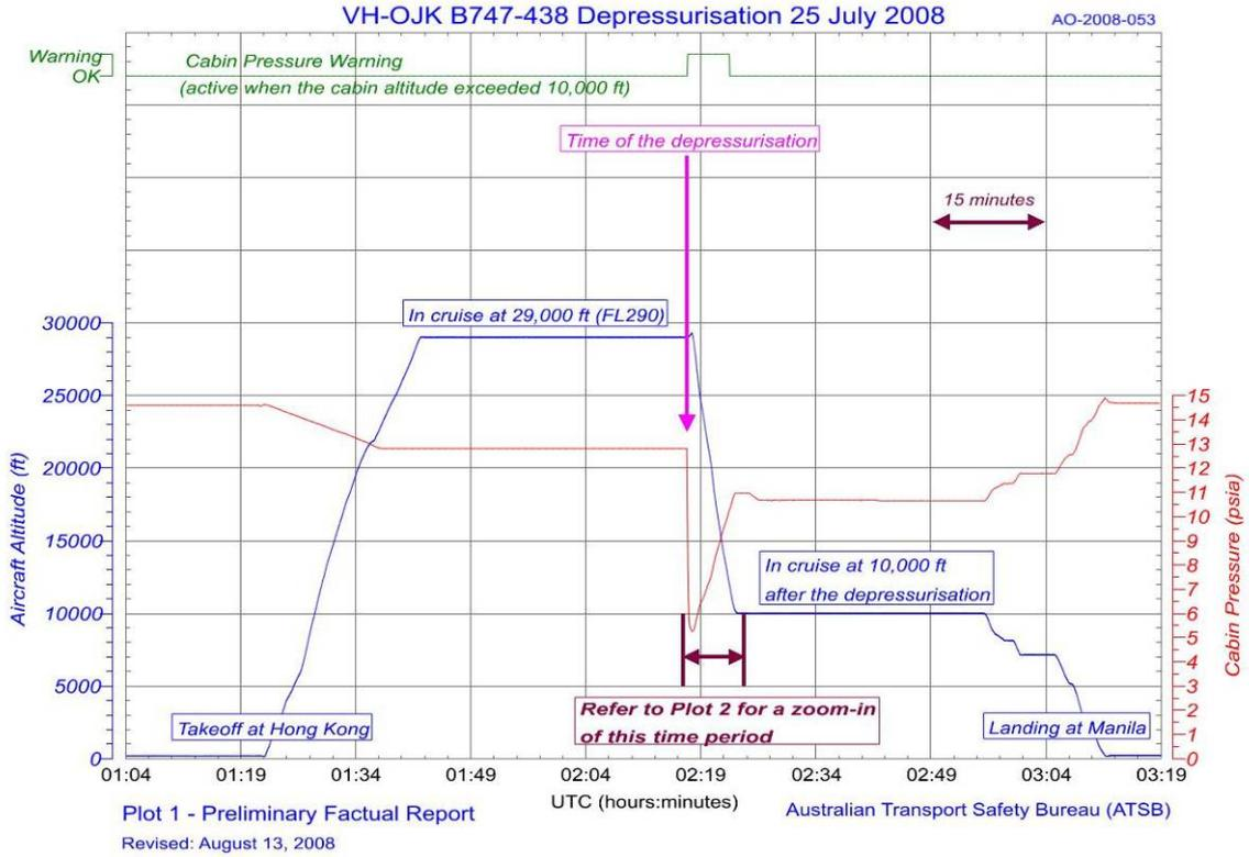
Figure C2: Data plot for the depressurisation event
