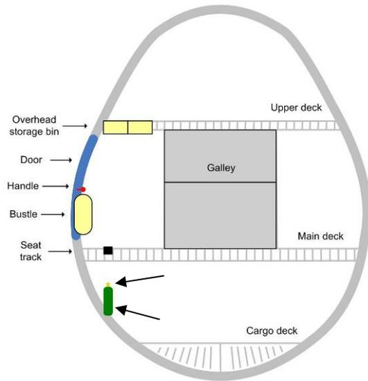
1. Normal arrangement (Oxygen cylinder and valve arrowed)
