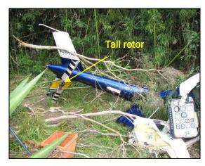
None of the occupants' seat belt attachment fittings were damaged. Examination of the wreckage did not indicate any mechanical defects that would have affected the safe operation of the helicopter.
