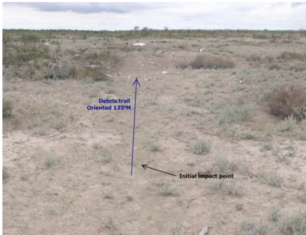
Figure 2: Initial impact point and debris trail
