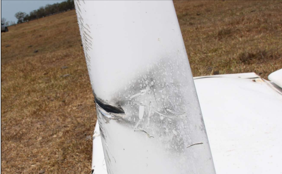
Figure 4 - Electrical arcing on strut
