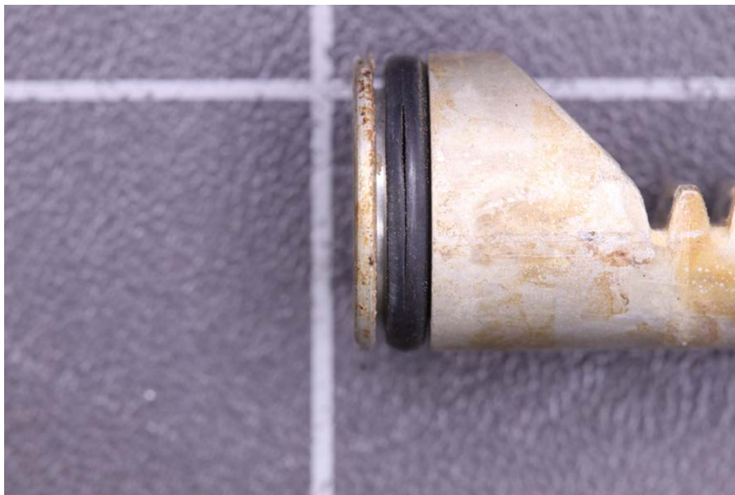
Figure 5: O ring deterioration
