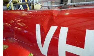
Damage to VH-XJA
