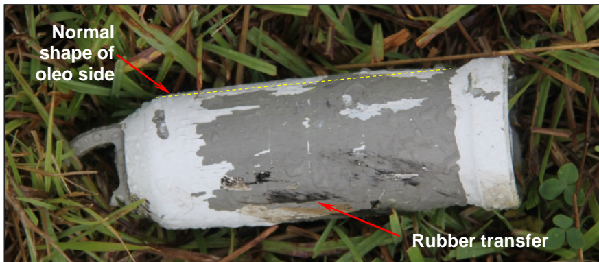
Figure 8: Left main landing gear oleo showing bulging
