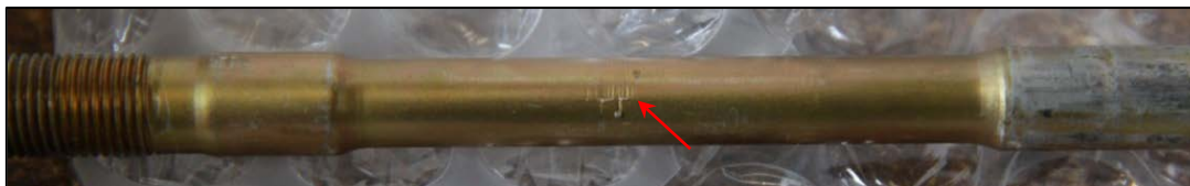
Figure 13: Gouging under the cadmium plating on one of the Continental through bolts (arrow)
