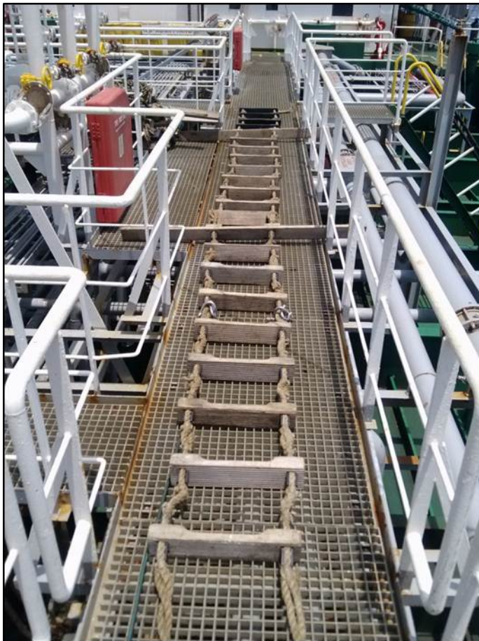
Figure 4. The pilot ladder laid out for inspection after the fall
