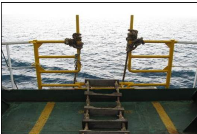
Figure 6. Manrope securing arrangements
