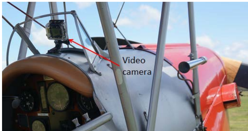
Figure 8: Mounting position of the recovered camera
