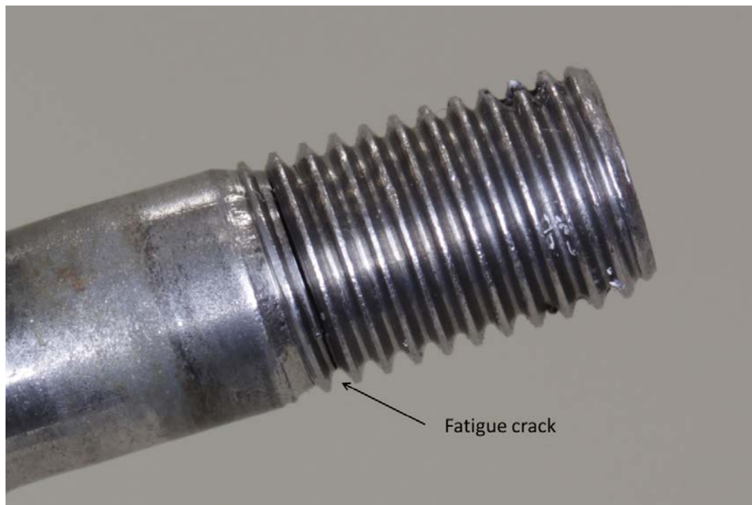
Figure 16: Forward fuselage lateral tie rod showing right side thread
