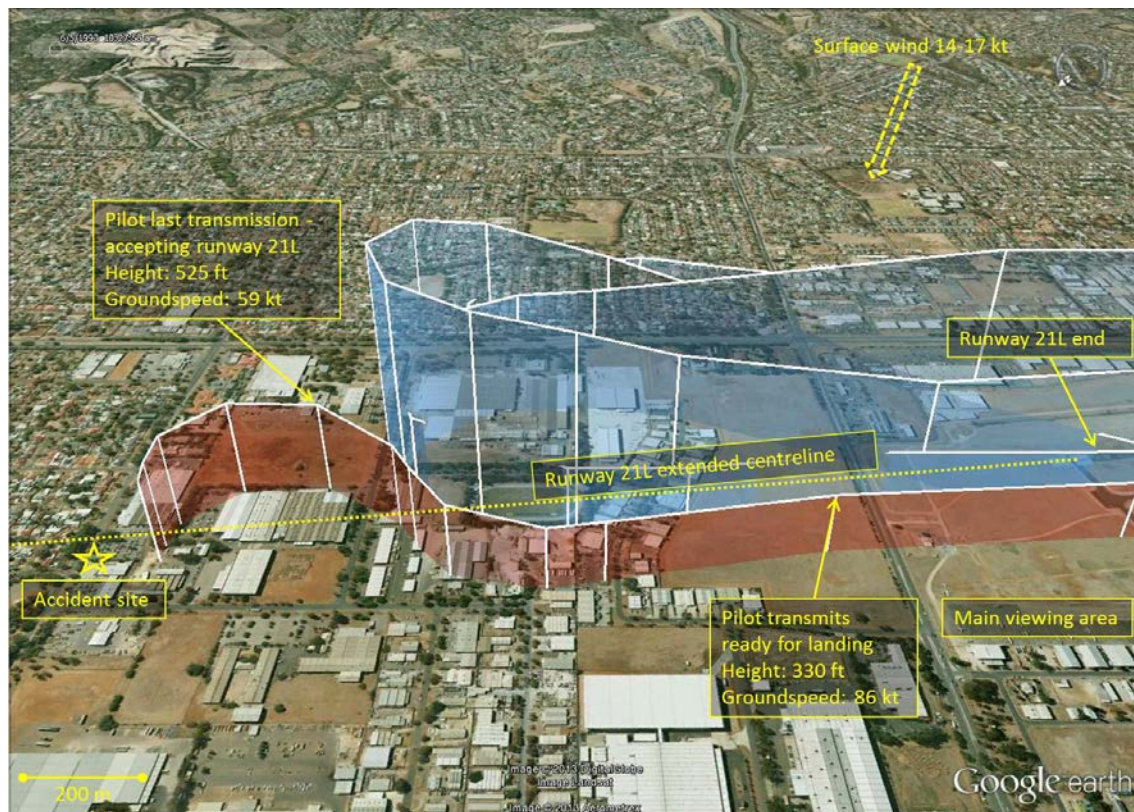
Figure 3: Spitfire GPS data re air display flight transposed onto satellite image (last fly-past and accident sequence highlighted red and prior display highlighted blue) with key events annotated
