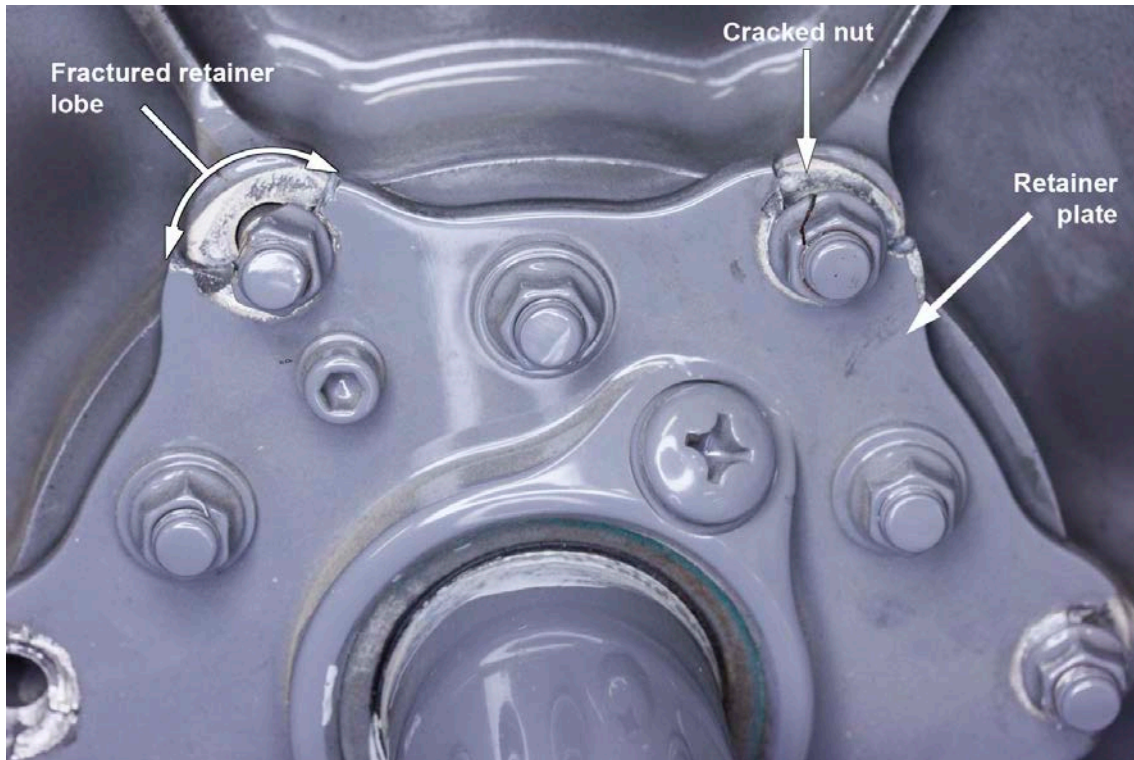
Figure 4: Close view of the clutch assembly damage. Five of the nuts had either cracked or had fractured.
