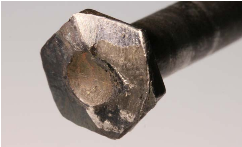
Figure 12: Worn head of a retention plate outer bolt from contact with the clutch actuator fixed bearing journal.
