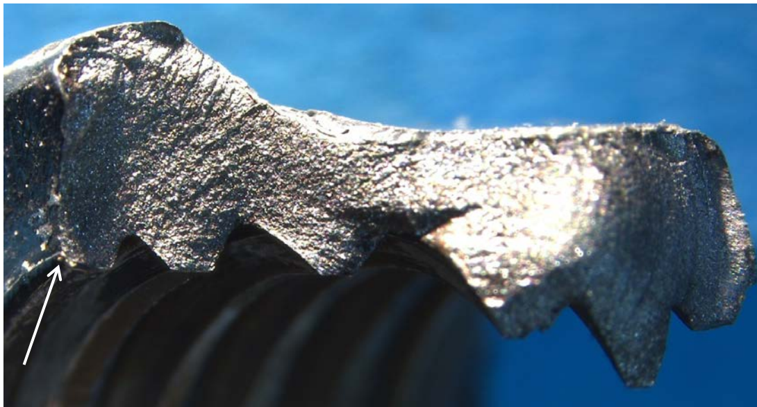
Figure 7: Typical, axially-orientated nut fracture surface; note the reflective grain facets
