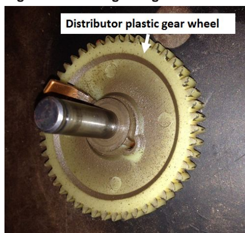
Figure 3: Left magneto gear wheel
