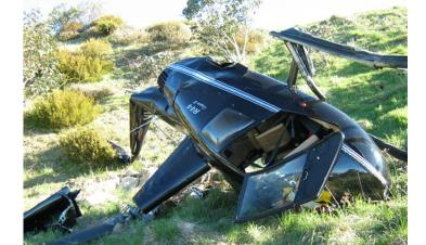
Figure 1: Damage to VH-UGC
