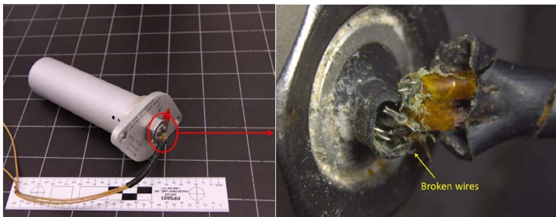
Figure 4: Low fuel float switch and faulty electrical connection
