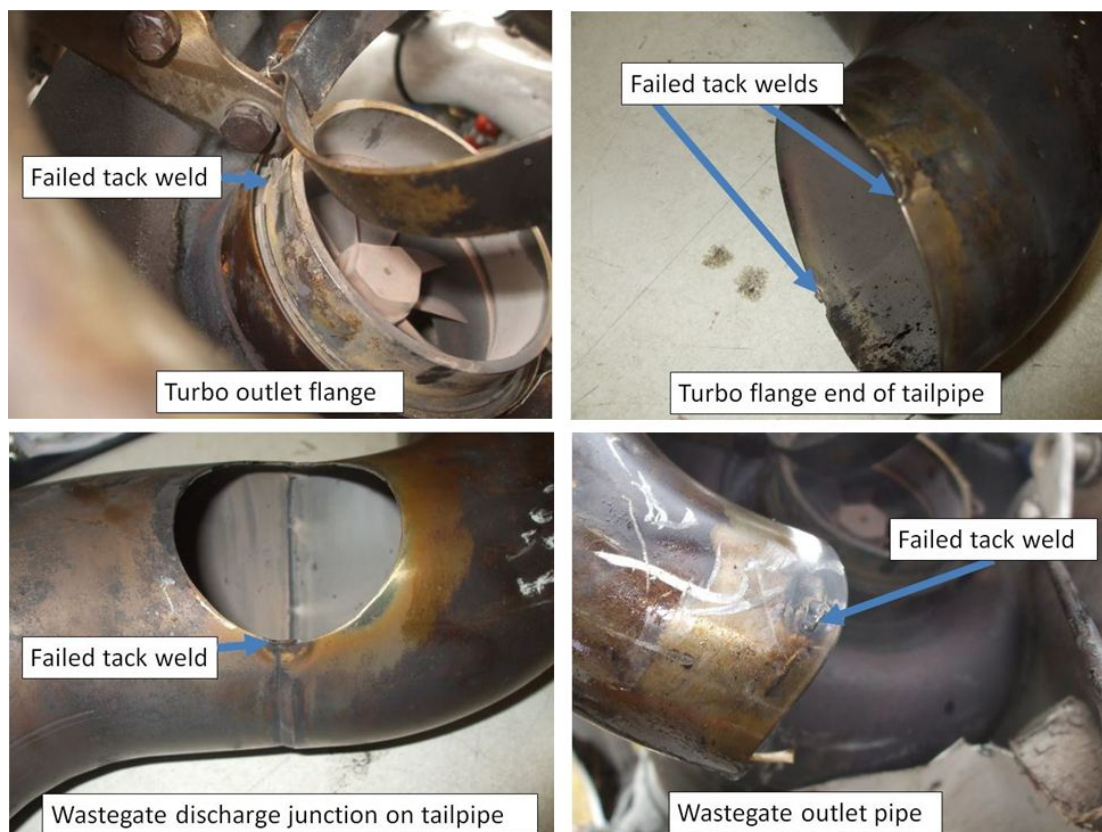
Figure 3: Failed tack welds
