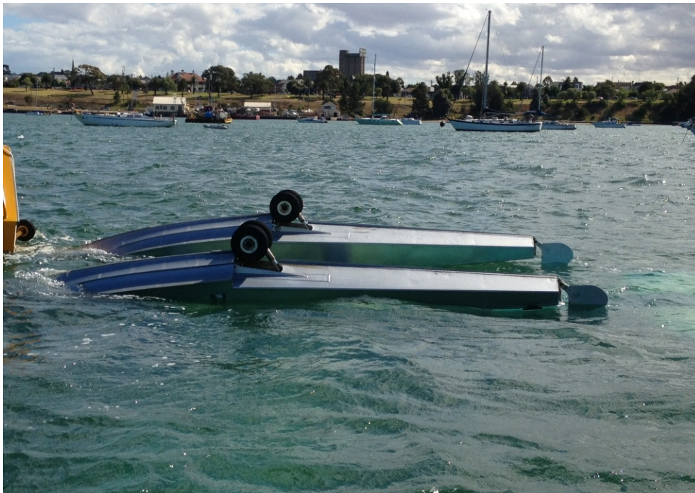
Figure 2: VH-UBI post-accident with the wheels extended
