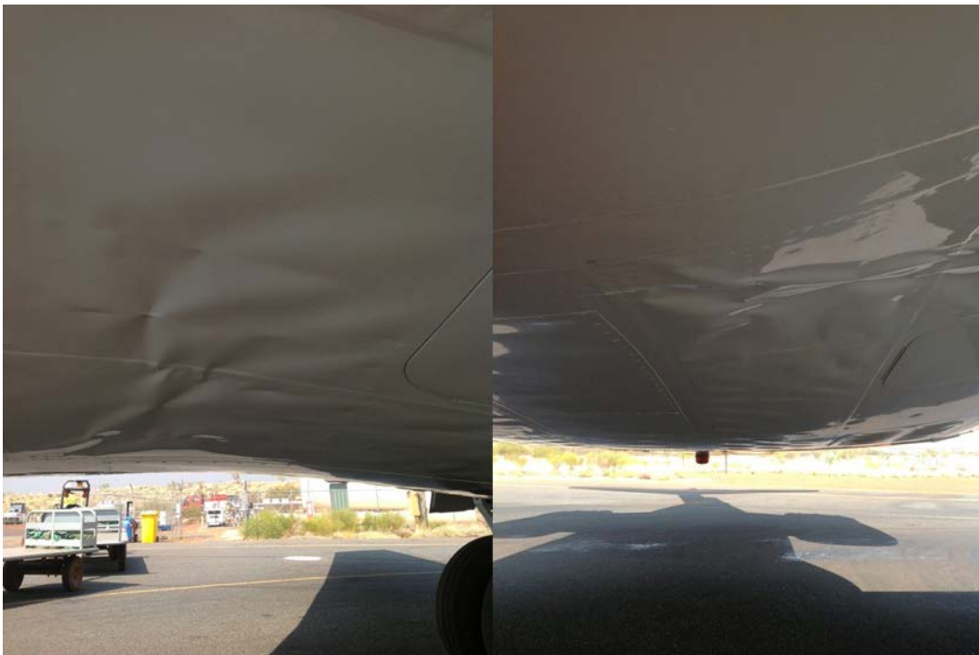
Figure 4: Aircraft skin damage, underbelly and centre section
