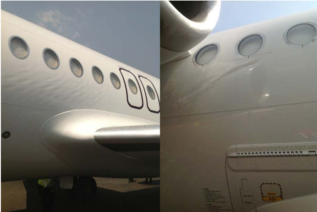
Figure 3: Aircraft skin damage, fuselage fore and aft
