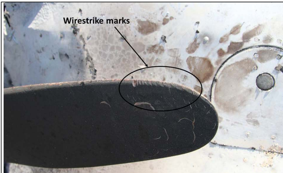
Figure 8: Propeller blade tip with wirestrike damage
