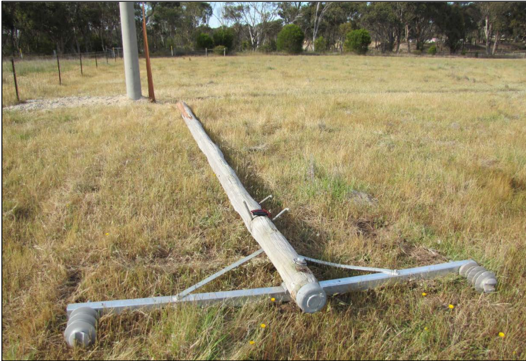
Figure 7: Broken power pole with the replacement pole in the background
